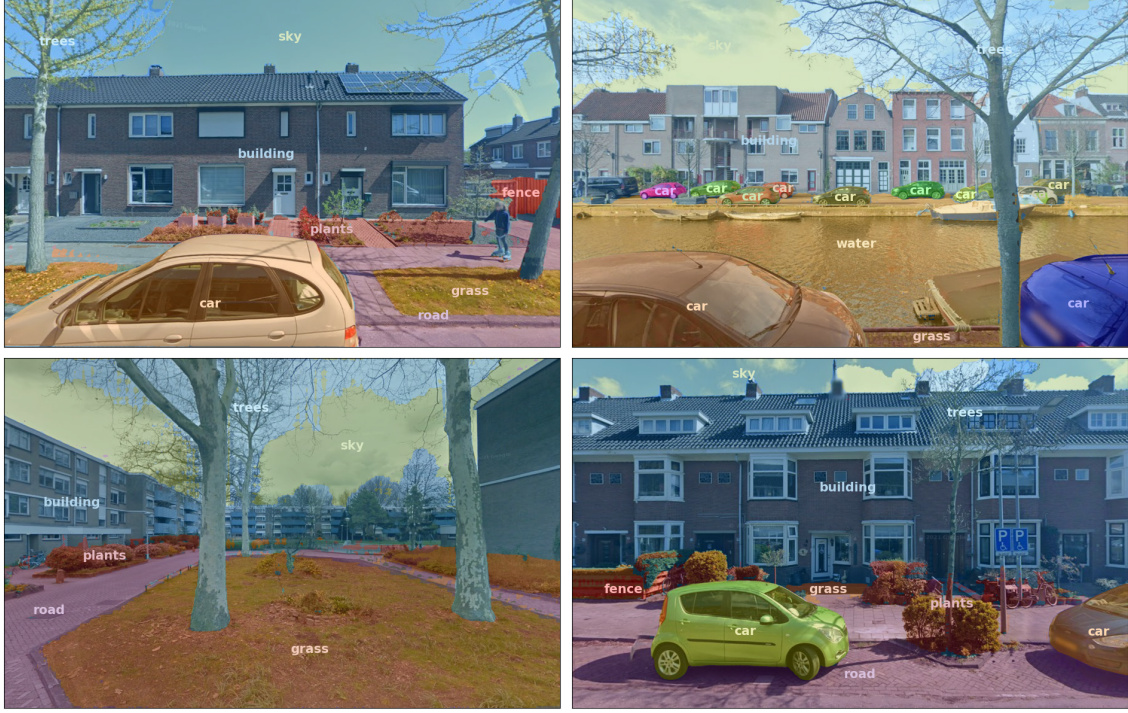
Figure 5: Four examples of segmented images using GroundingDINO and SAM
