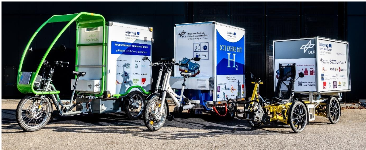
Figure 1: Three examples of the trialed fuel cell cargo pedelecs: Bring S by Bayk, UM CargoBike by Urban Mobility, Amadillo by Velove (photo: DLR)
