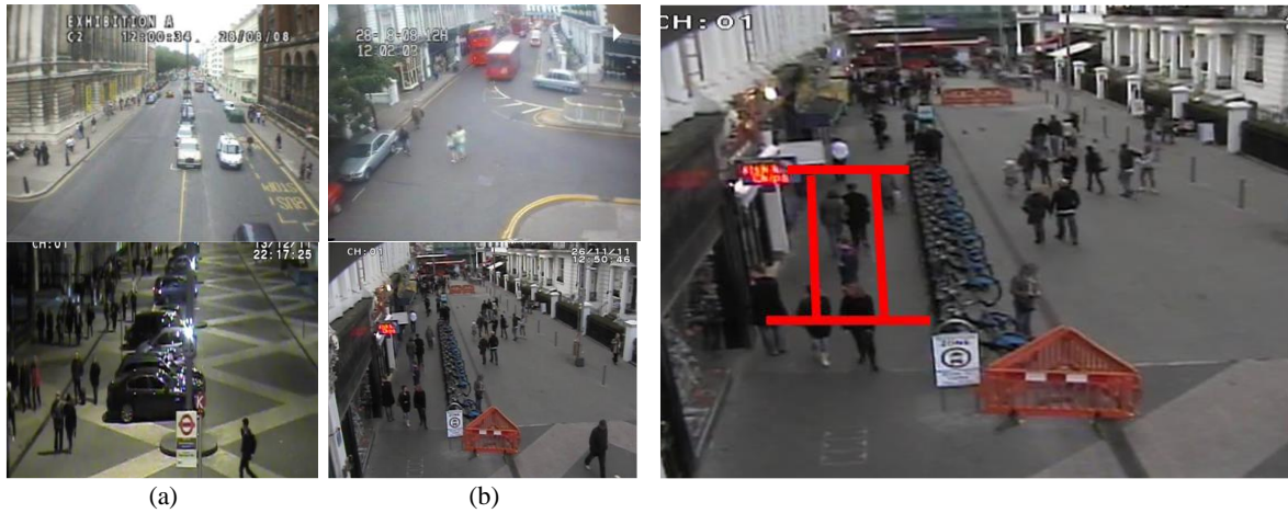
FIGURE 4: (Left) examples of footage used – before (top) and after (bottom) the re-design: (a) Exhibition Road (L1), (b) Thurloe Street (L4); (Right) “bottleneck” method for extracting pedestrian traffic measurements.
