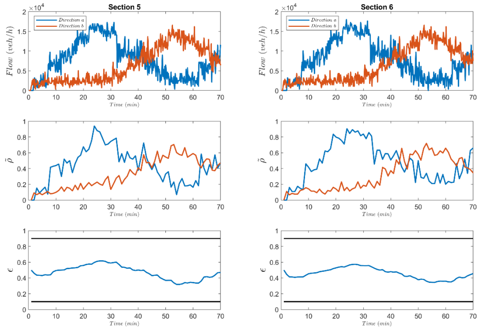
Fig. 8: Flow, relative density and control input for the IBC case (Section 5 & 6)
