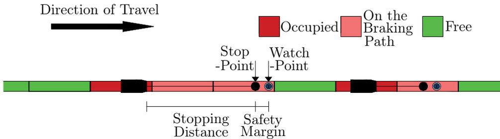
Figure 1: Simulation concepts. The train’s watch-point (eye symbol), stop-point (black circle), stopping distance (horizontal black line), and the block states differentiated by colour. Blocks on the braking path are reserved so that other trains may not enter them.
