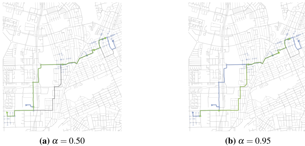
Figure 5: The route of a door-to-door pooled ride with three travellers, visualised in blue, and the new route with PUDO points in green, when using different service settings \alpha .
