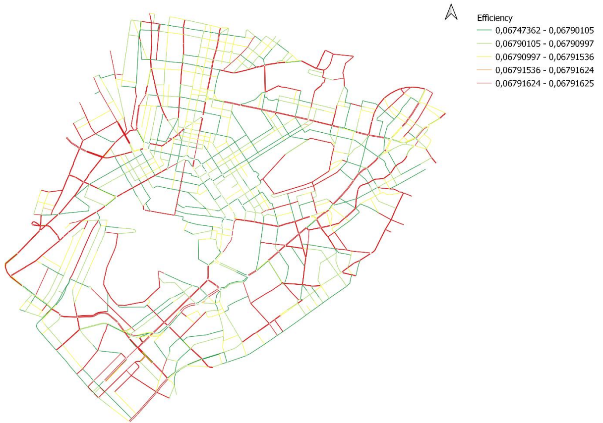
Figure 3: Efficiency after the removal of each link from graph G.
