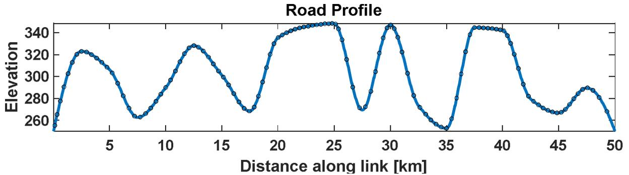
Figure 1: Road profile versus link distance (note vertical axis in m, horizontal in km). Dots mark 30s timesteps.
