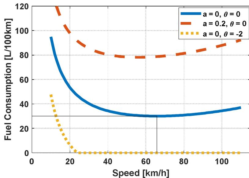
Resulting fuel consumption curves (litres/100km) are shown below. Optimal cruising speed is marked [65.72km/h]. Note instantaneous fuel consumption is bounded below by zero. To illustrate the importance of capturing acceleration and within-link gradient, we consider an undulating link of length 50km with zero net gradient i.e. link-ends have the same elevation. Our example elevation profile is randomly generated, inducing a maximum gradient of 3.16 degrees.
