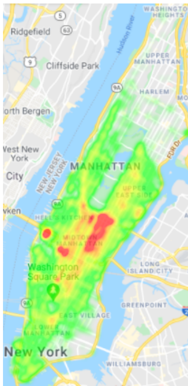
Fig. 3. Departure rate at each node in the graph. Red dots generate more requests.
