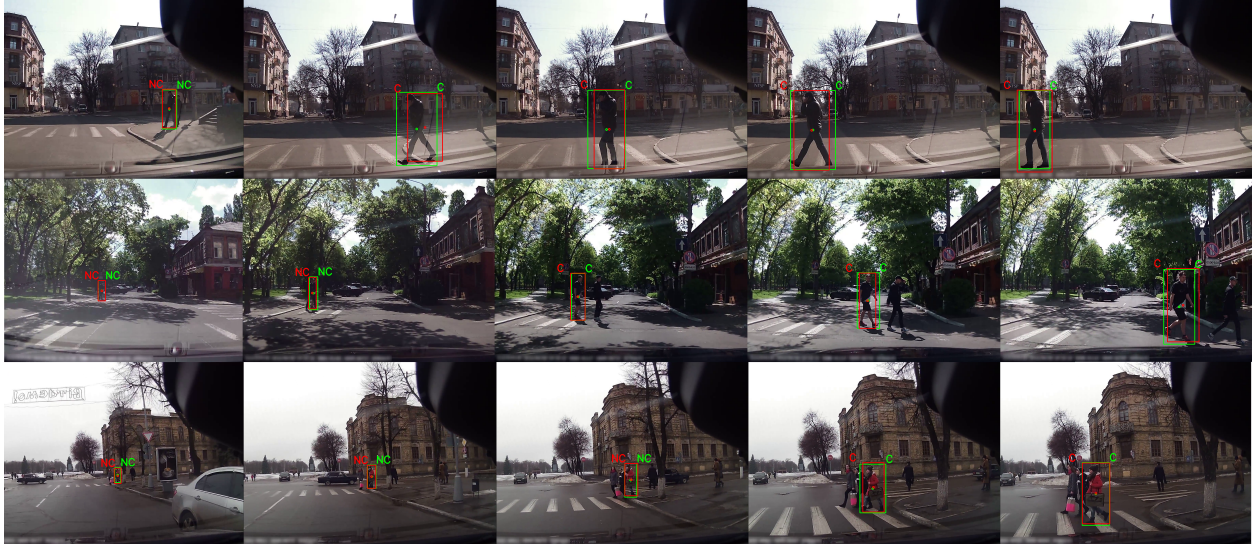
Figure 2: Visualisation of the pedestrian bounding box and intention prediction in different scenarios. Red rectangle/text: Predicted bounding box/intention | Green rectangle/text: Ground truth bounding box/intention | C : Crossing | NC: Non crossing. Each frame represents a time step, going from left to right. The first row shows how our model acts at points where the state of the pedestrian changes from crossing to non-crossing. The second shows a whole crossing sequence. The third shows how our network handles non-moving pedestrians when the car is moving.
