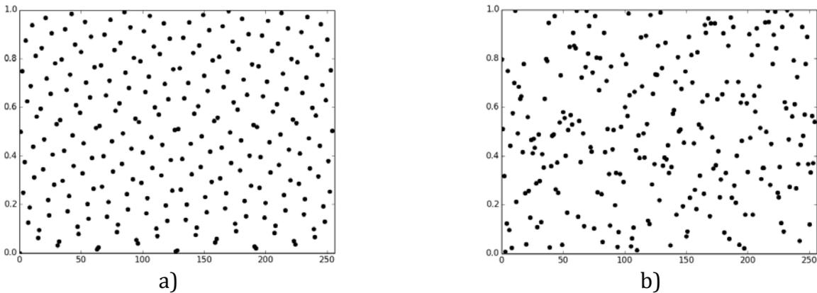
Figure 2. Realizations or random numbers: Sobol (a) versus Mersenne Twister (b)
