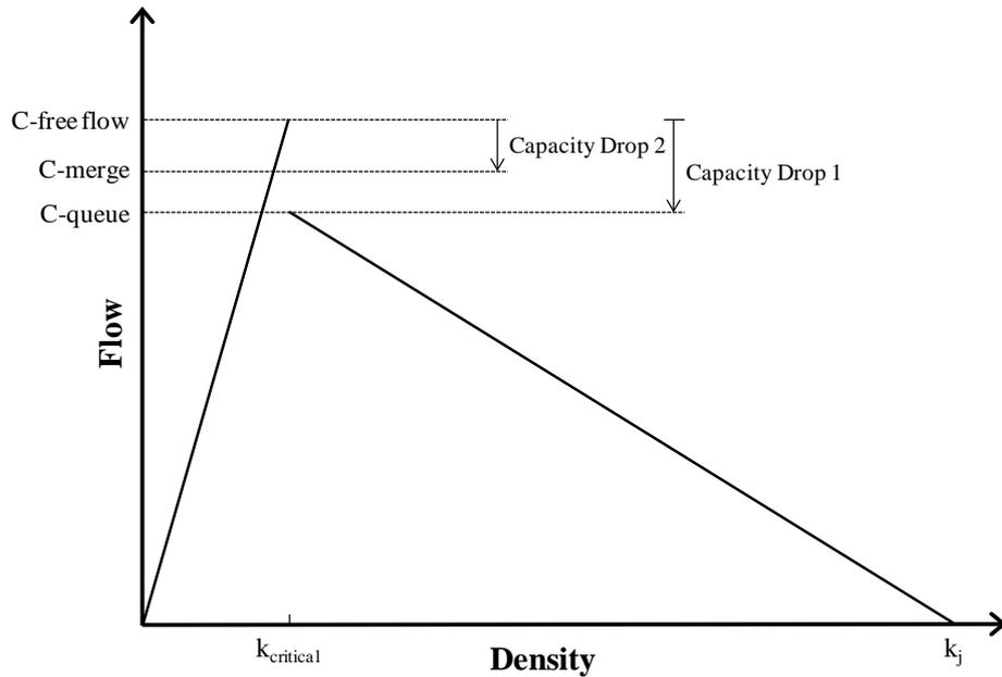
**Figure 1** Inverse-lambda shaped fundamental diagram
