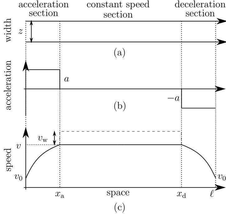
Figure 1: Accelerating moving walkway characteristics: (a) width profile, (b) acceleration profile and (c) speed profile over space.
