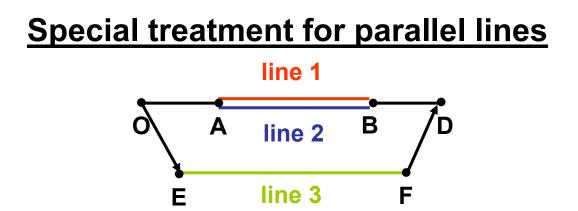
In such a case, one does not consider 2 different paths O-A-B-D, but only one path with the combined line (1+2)
