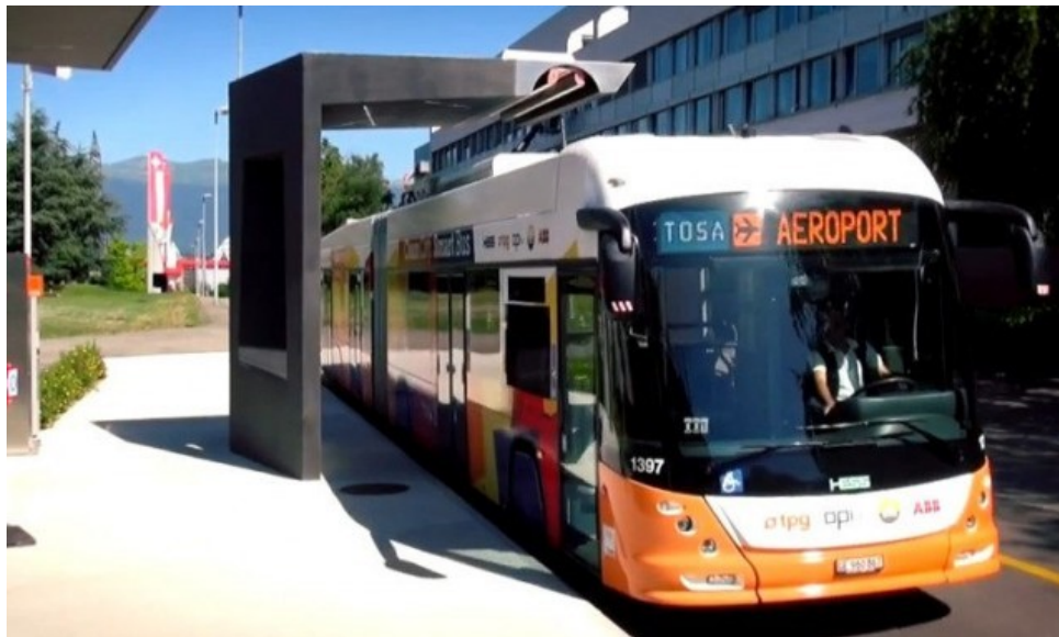
Figure 2: TOSA bus and wayside feeding station
