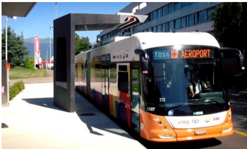
Figure 2: TOSA bus and wayside feeding station
