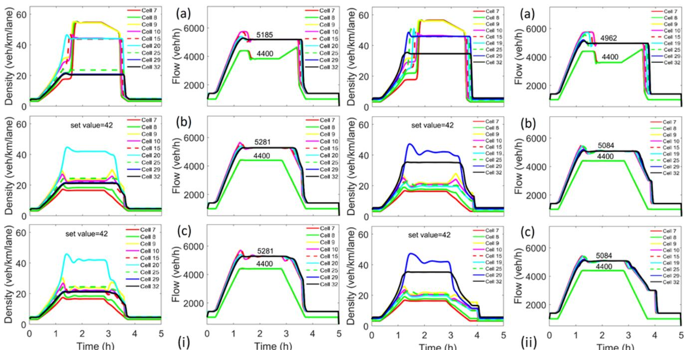
Fig. 2: (i) Bottleneck case 1: (a) no control, (b) LQI, (c) PI-ALINEA, (ii) Bottleneck case 2: (a) no control, (b) LQI, (c) PI-ALINEA
