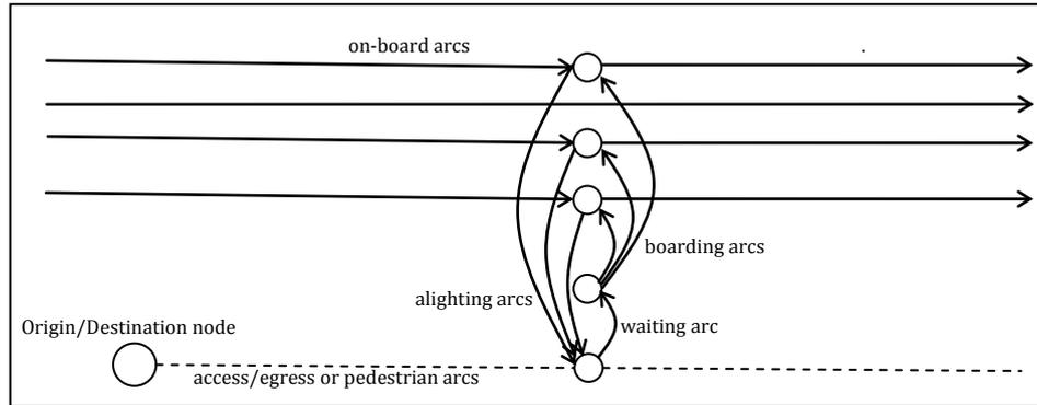
Figure 1. Arcs and nodes modelling a bus stop
