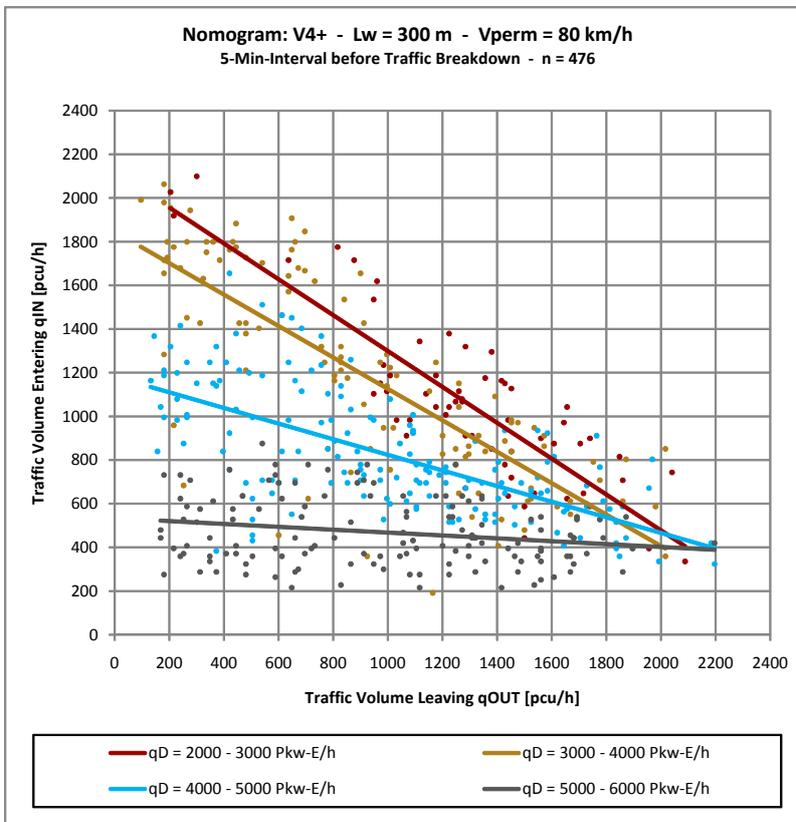
Figure 4: Two examples for V3 and V4+ nomograms
