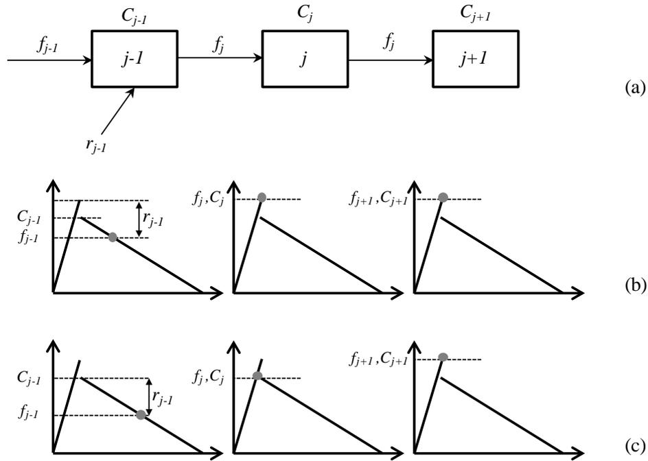
**Figure 2** (a) Cells configuration indicating its capacity (“C”), entering flow (“ $f$ ”) and on-ramp rate (“ $r$ ”), if exists. Current flow and available capacity of each cell (c) considering and (b) without considering capacity drop in cell “ $j$ ”.
