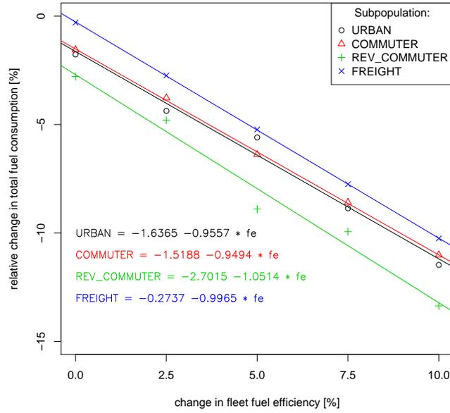
Figure 3: Impacts of fuel efficient cars on fuel reduction:
