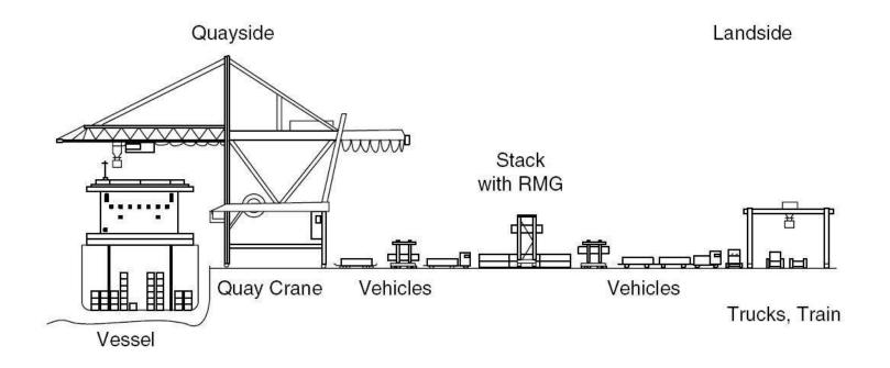
Scheme of a container terminal system (Steenken et al., 2004).
