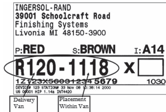
Figure 2. A preload assist label identifies the delivery van that is assigned to a package and specifies where to place it in the delivery van.
